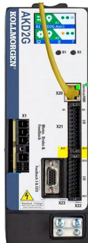
Confirm that the link LEDs on the drive (green LED on the RJ45 connector) and on your PC are both illuminated. If both LEDs are illuminated, then you have a working electrical connection.
